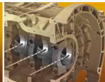
7 Alésage des trous de lubrification vilebrequin Boring of lubrication holes for crankshaft
